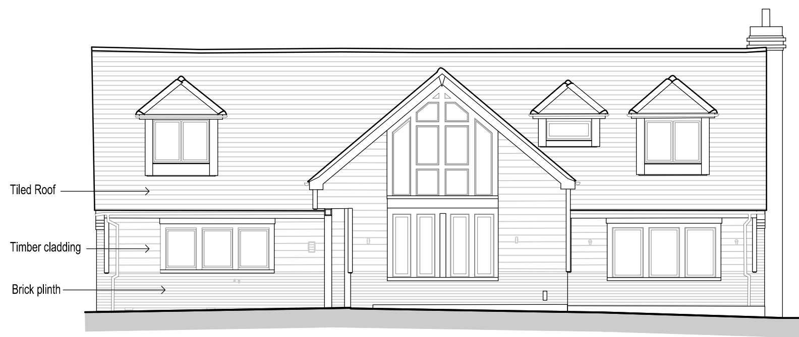
North West Elevation
